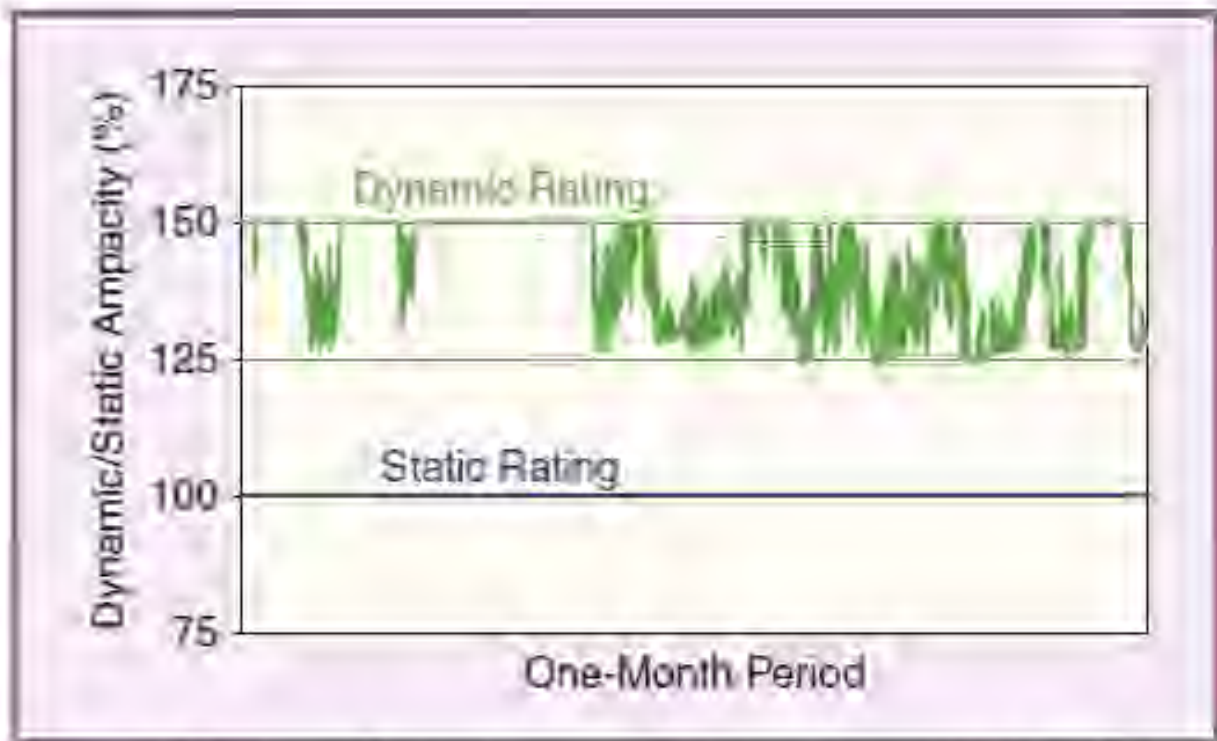
Figure 16. The dynamic current rating compared with the static rating over one month for TenneT OHLs.
